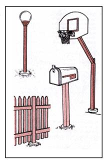
strength buildup. Consider that when placed in a hole or dirt form, water can be sucked out of the concrete by the surrounding soil. This shortens curing time and reduces concrete strength. For this reason, many local building codes now specify the use of forms for all footers and foundations used in load-bearing applications.
