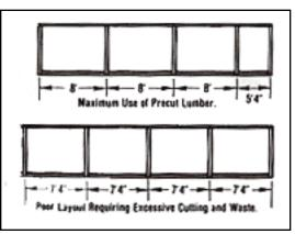
3. To find the exact post locations, mark both end points of the fence with wooden stakes and run a line between them. Locate positions for all posts between the end posts by measuring intervals with a tape, or by laying out the precut rails in line along the ground.
